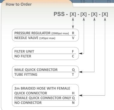
**NOTE:** PSS comprises the system chassis, two bulkhead connectors and piping for connection to the instrument, flow indicator and connecting piping to the instrument outlet bulkhead. An anti-static carrying case is included.
